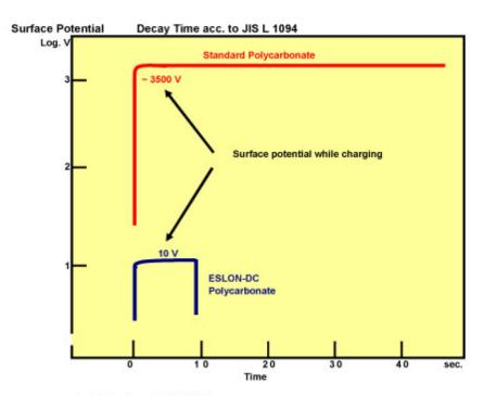
Test Method acc. to JIS L1094
