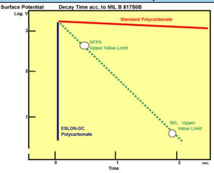
Test Method acc. to MIL B 81750B
